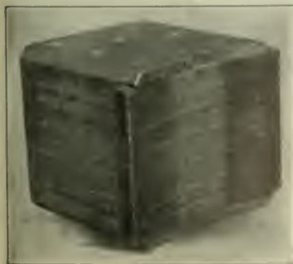
FIG. 2. MAGNET CORE OF WESTINGHOUSE MOTOR
